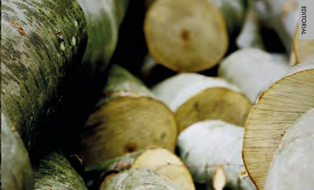
The impact of wood moisture on combustion quality is often massively underestimated by residential fireplace users. The negative effects of this include poor efficiency, lower heating output, more quickly soiled panes, more pollutants and sooting of the exhaust system.
